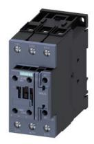
power contactor, AC-3e/AC-3, 41 A, 18.5 kW / 400 V, 3-pole, 110 V AC, 50 Hz, auxiliary contacts: 1 NO + 1 NC, screw terminal, size: S2  $\,$
