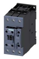
power contactor, AC-3e/AC-3, 65 A, 30 kW / 400 V, 3-pole, 110 V AC, 50 Hz, auxiliary contacts: 1 NO + 1 NC, screw terminal, size: S2  $\,$
