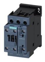
power contactor, AC-3e/AC-3, 9 A, 4 kW / 400 V, 3-pole, 110 V AC, 50 Hz, auxiliary contacts: 1 NO + 1 NC, screw terminal, size: S0  $\,$
