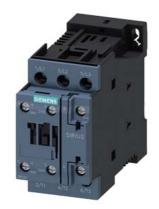
power contactor, AC-3e/AC-3, 9 A, 4 kW / 400 V, 3-pole, 24 V DC, auxiliary contacts: 1 NO + 1 NC, screw terminal, size: S0  $\,$
