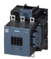
Power contactor, AC-3 150 A, 75 kW / 400 V AC (50-60 Hz) / DC operation 220-240 V UC Auxiliary contacts 2 NO + 2 NC 3-pole, Size S6 Busbar connections Drive: conventional screw terminal
