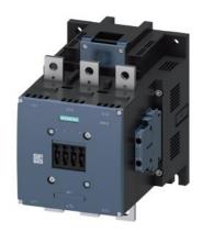
Power contactor, AC-3 400 A, 200 kW / 400 V AC (50-60 Hz) / DC operation 220-240 V UC Auxiliary contacts 2 NO + 2 NC 3-pole, Size S12 Busbar connections Drive: conventional screw terminal
