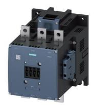
Power contactor, AC-3 500 A, 250 kW / 400 V AC (50-60 Hz) / DC 220-240 V UC Auxiliary contacts 2 NO + 2 NC 3-pole, size S12 Busbar connections Operating mechanism: conventional screw terminals
