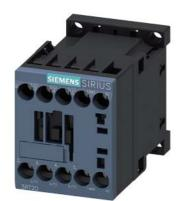
Power contactor, AC-3 16 A, 7.5 kW / 400 V 1 NO, 230 V AC, 50/60 Hz 3-pole, Size S00 screw terminals
