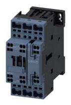
power contactor, AC-3 25 A, 11 kW / 400 V 1 NO + 1 NC, 230 V AC, 50 Hz 3-pole, Size S0 Spring-type terminal
