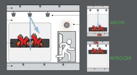
The IG-55 agent has unique properties that optimize its action: stratification of agent at various levels (argon, more dense than air, in the middle and lower parts, and lighter nitrogen above) provides comprehensive protection throughout the enclosure, minimizing possible leaks.
