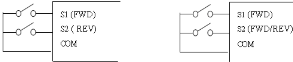
Figure 4-4 Terminal Board Drive Operation Modes
