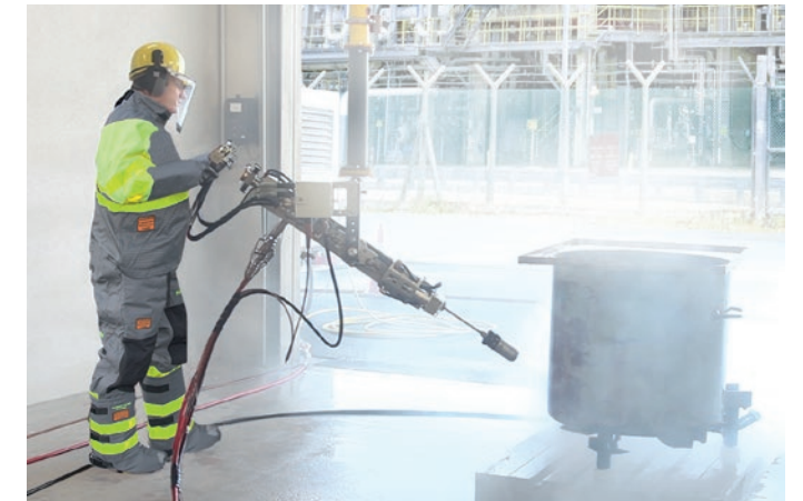
Jetmate - reaction force free jetting tool
