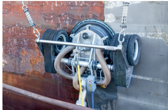
Spiderjet M - magnetically adhering surface cleaning device
