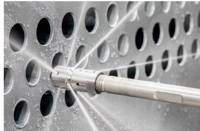
Nozzles for heat exchanger cleaning
