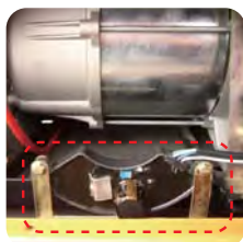
Window for AVR regulation Allows easy acces for After Sales
