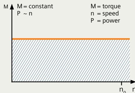
**High Overload (HO)** is generally used for applications demanding a higher dynamic performance (cyclic duty), as well as constant torque characteristics with a high breakaway torque.
