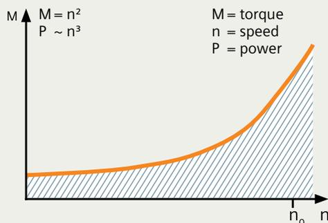
**Low Overload (LO)** is generally used for applications demanding a low level of dynamic performance (continuous duty), square-law torque characteristic with low breakaway torque and low speed precision.
