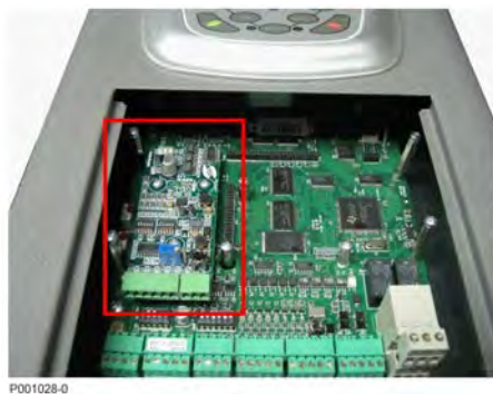
Figure 124: Encoder board fastened to its slot
