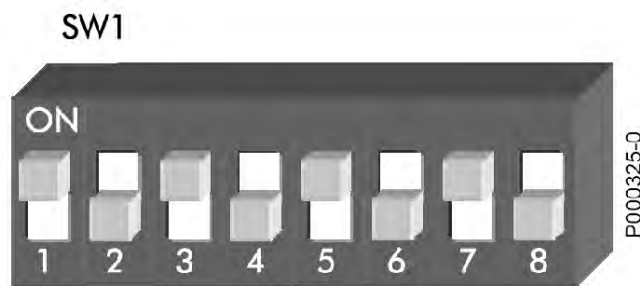
Figure 188: DIP-switch SW1 setting in three-channel mode
