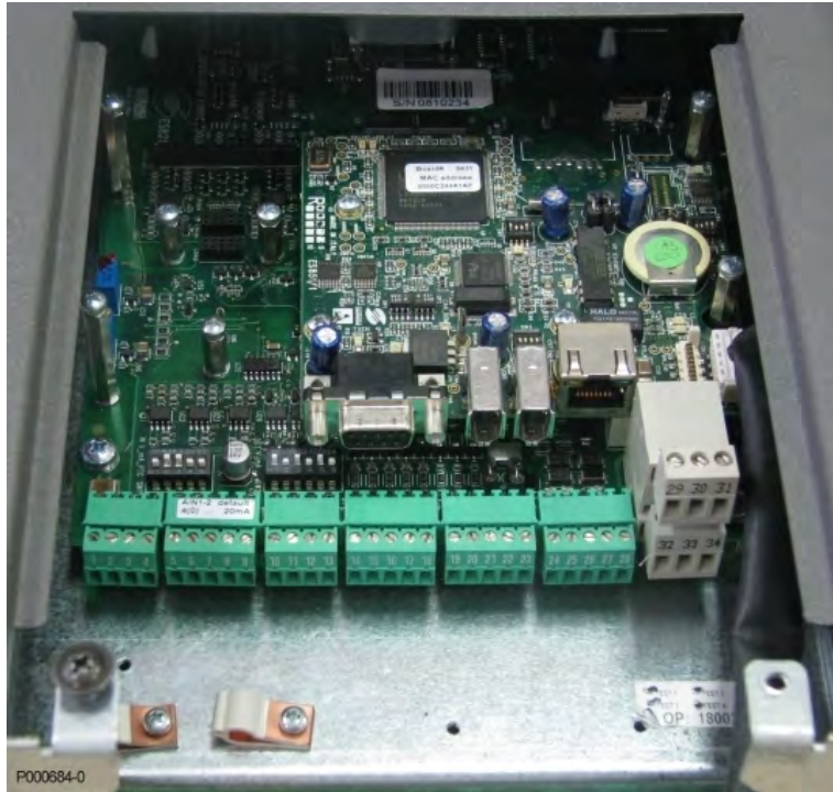
Figure 159: ES851 DataLogger fitted into slot B
