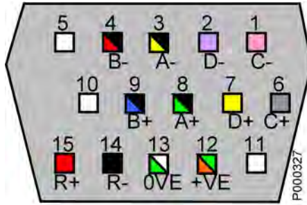
Figure 187: Pin layout on the high density connector
