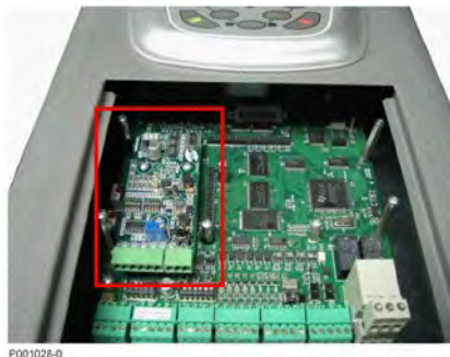
Figure 115: Encoder board fastened to its slot
