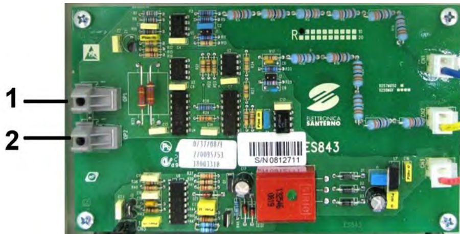
Figure 37: ES843 Bus-bar Voltage Acquisition Board
