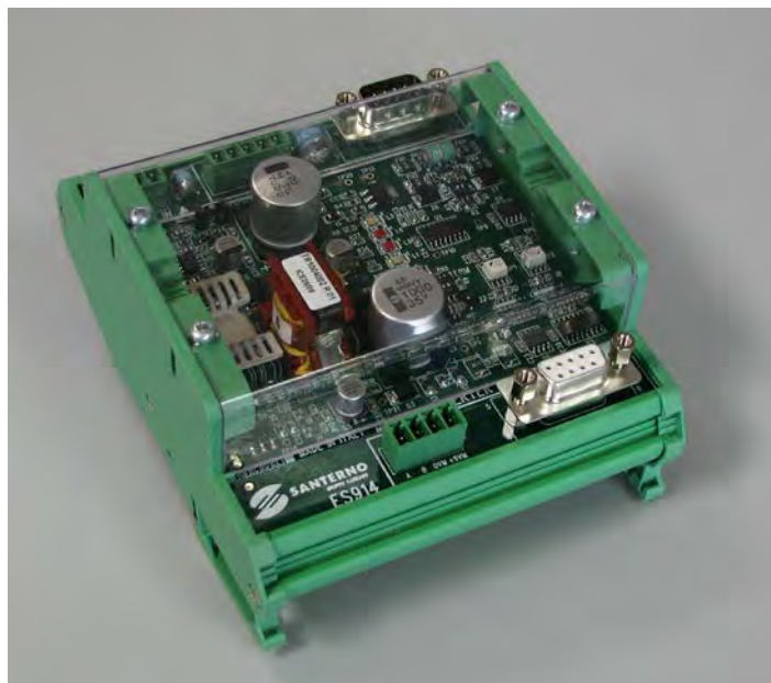
Figure 179: ES914 Power supply unit board
