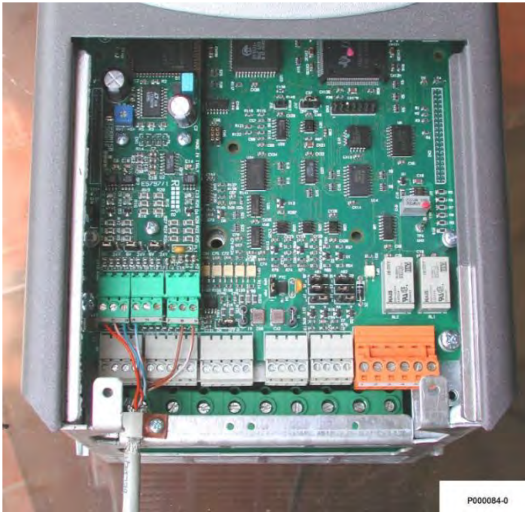
Figure 121: Wiring the encoder cable
