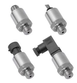
PCM390 pressure transmitter is specially designed for small and medium equipment applications such as booster pumps and air compressors. It is also applicable to a wide range of industrial applications, with a variety of structures, output forms and pressure connections to meet the requirements of most applications. PCM390 is designed with compact structure which especially applies to the installation in small space.
