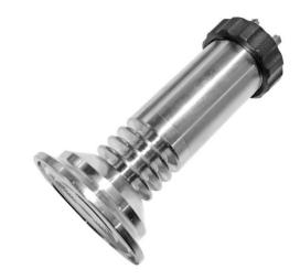
PCM1350 flush pressure transmitter is applicable to food, beverage, pharmaceutical and biological engineering. Full metal flush-mounting isolation diaphragm is directly welded with process connection to ensure the precision connection between process connection and measuring diaphragm. Therefore, no additional sealing gaskets are required, and it ensures there are no measurement dead zones.
