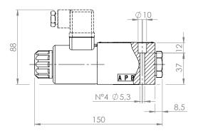
All valves HD3-\* conform with ISO and CETOP specifications for mounting surface dimensions (see 9) and for valves height. When assembled to its mounting plate valve HD3-\* must be fastened with 4 bolts M5x45 (or M5x\*\* according to the number of modules) tightened at 8 Nm torque. Leakage between valve and mounting surface is prevented by the positive compression on their seats of 4 seals of Quad Ring type 9,25x1,68x1,68.
