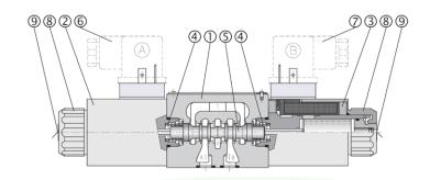
The spool 5 shifts into the valve body 1 subject to the action of springs 4 and solenoids 2. Spool 5, depending from its shape and its position in the valve body, opens and/ or closes passages between P, A, B and T ports, thus controlling the direction of the hydraulic flow.
