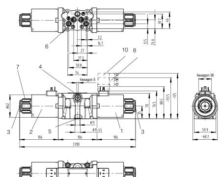
All valves HD5-ES-\* conform with ISO and CETOP specifications for mounting surface dimensions and for valves height.
