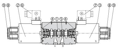
The spool 1 shifts into the valve body 7 subject to the action of springs and solenoids 2 and 3. Spool 1, depending from its shape and its position in the valve body 7, opens and/or closes p assages b etween P, A, B and T ports, thus controlling the direction of the ydraulic flow. In case of electric cut-offs the spool can be manually shifted by acting on the override pins 9, located at the end of the solenoids and accessible through the retaining nuts.
