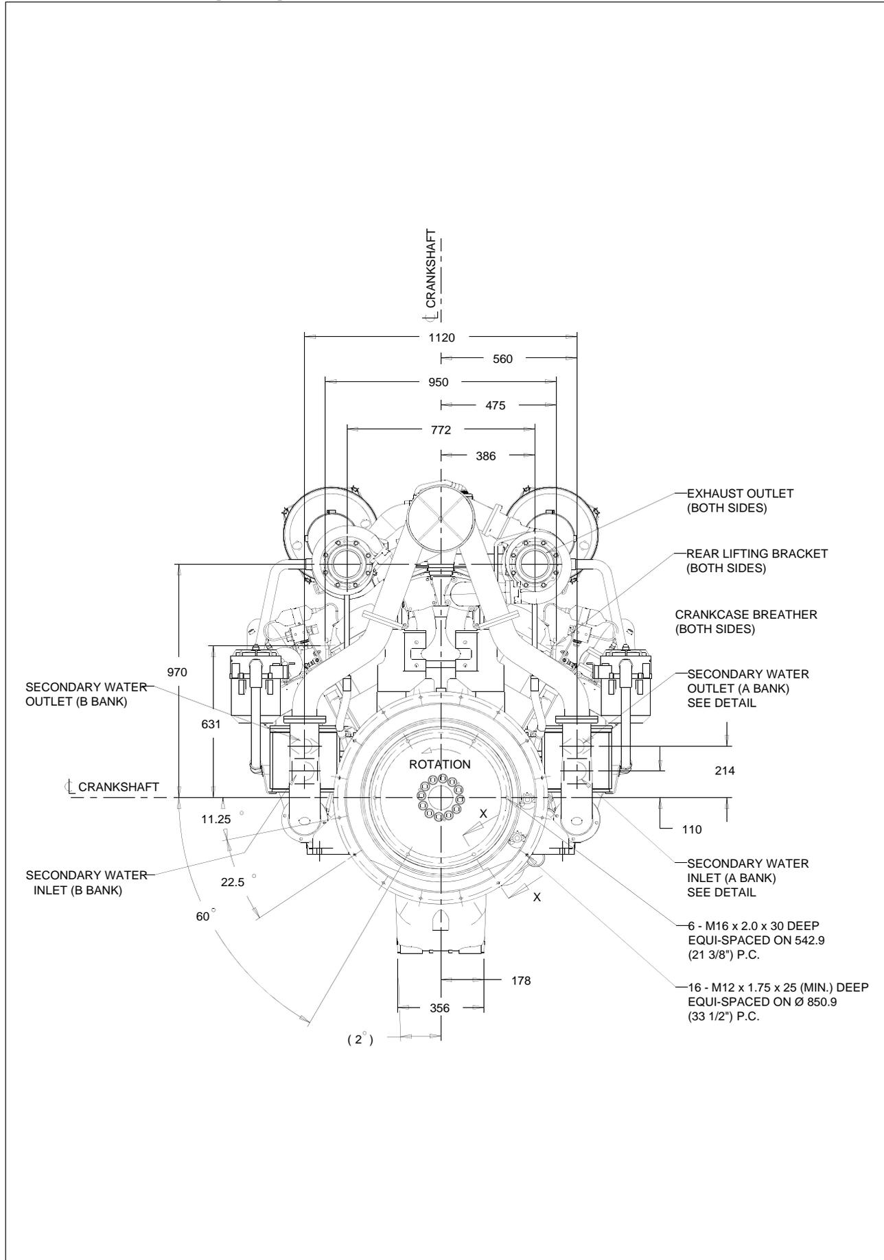
**4016-61TRS1&2 Natural gas co-generation - SAE Flywheel, Exhaust Outlet and Support Pads**
