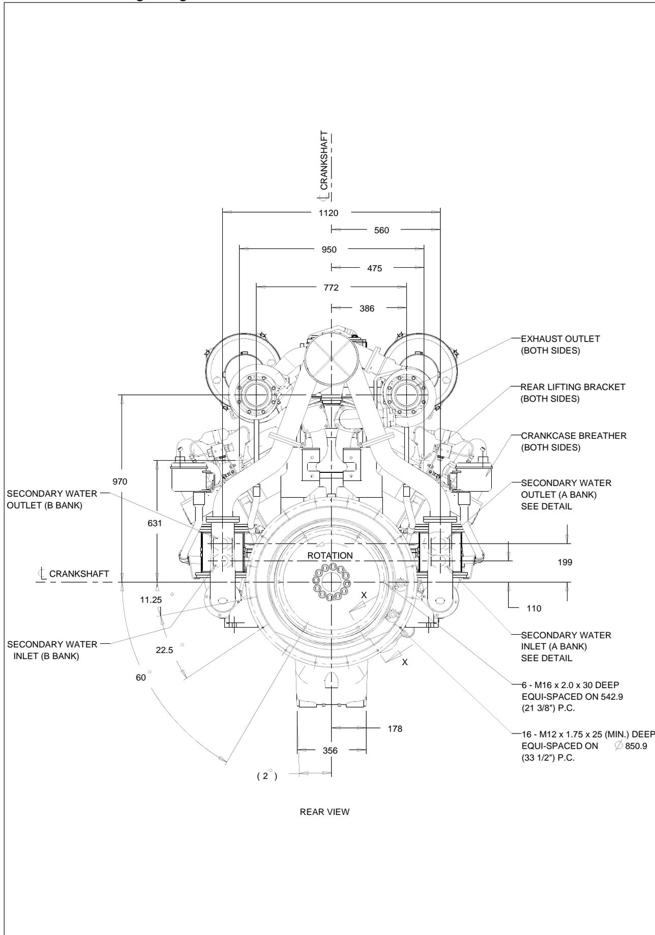
**4016-61TRS1&2 Bio gas cogeneration unit - Electrical connections, Exhaust Outlet and**
