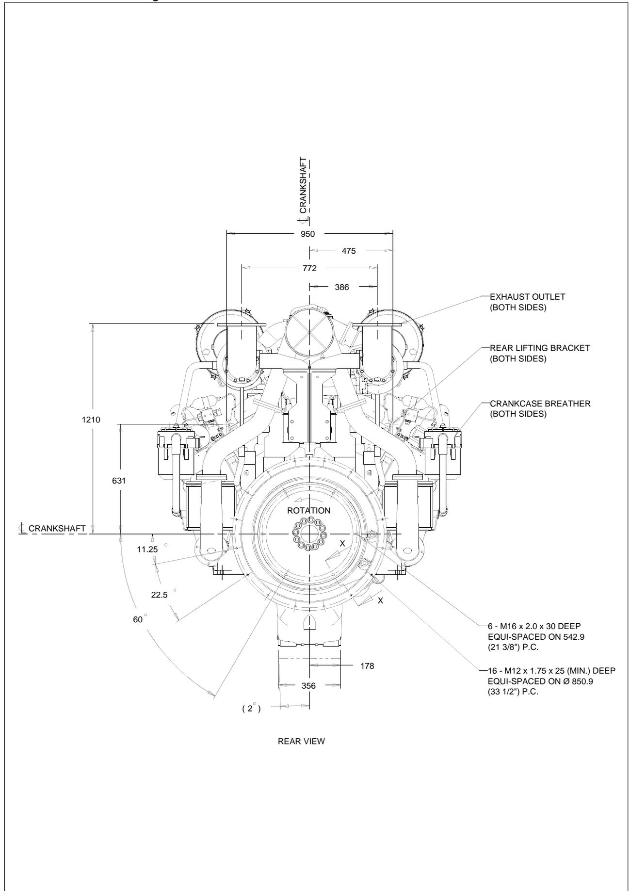
**4016-61TRS1&2 Natural gas electro unit - SAE Flywheel, Exhaust Outlet and Support Pads**
