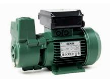
Self-priming peripheral pump with star impeller, with a great suction capacity. Cast iron body with brass ring. Motor support and impeller in brass to avoid the risk of blocking. Driving shaft in stainless steel. Carbon/ceramic mechanical seal.
