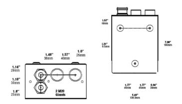
Leave 3.14" (80mm) clearance at top and bottom of docking station for access.
