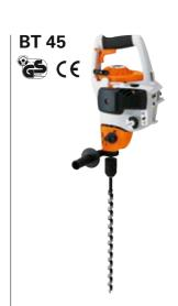
27.2 cm<sup>3</sup>, 0.8 kW/1.1 hp, 4.8 kg\*. Hand-held drill with powerful petrol engine for drilling wood. Standard with two-speed gearbox, reverse gear for releasing jammed drills and neutral position. Available with quick-release chuck with a chuck width of 13 mm.
