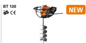
36.3 cm<sup>3</sup>, 1.4 kW/1.9 hp, 9.9 kg\*. High-torque one-man auger, 4-MIX® engine with low fuel consumption, low noise and vibration levels, standard with QuickStop drill brake, long-life air filter system, support cushion.
