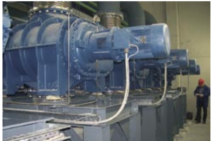
▲ 4-stage vacuum plant with 2 x 30.000 m 3 /h intake volume in steel degassing ▼
