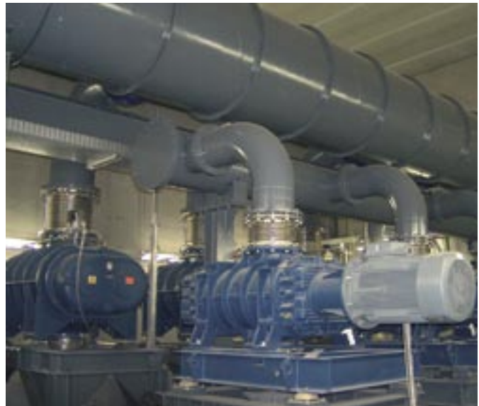
▲ 4-stage vacuum plant with 2 x 30.000 m 3 /h intake volume in steel degassing ▼
