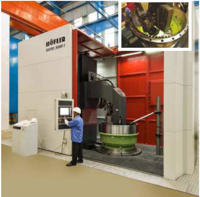
Profile Grinding Machine (Internal / External – 3000 mm Dia)
