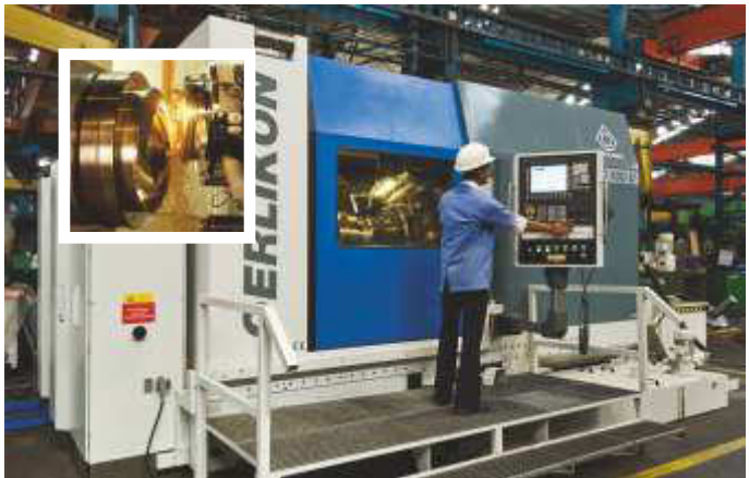
Spiral Bevel 'Hard Cut' Machine (1100 mm Dia)
