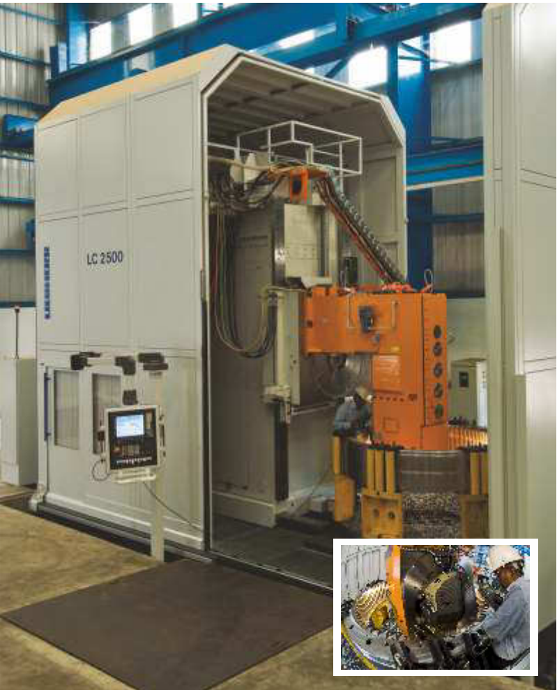
Gear Hobbing Machine (Internal / External – 2500 mm Dia)
