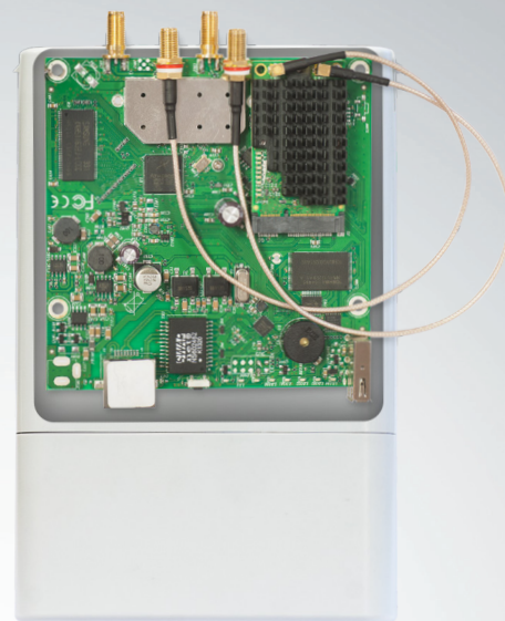
Rendered image shows internals of BaseBox with optional second wireless card
