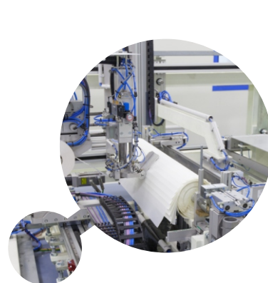
Automatic and manual rolling of spiral wound elements
