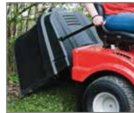
Almost all tractors with rear discharge have a grass catcher which is easy to empty from the driver's seat
