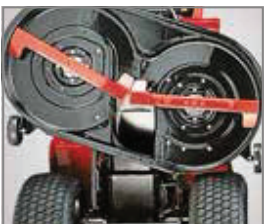
Tractors with rear discharge and a two-blade system have counter-rotating blades which
