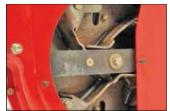
Specially hardened self cleaning steel blades
