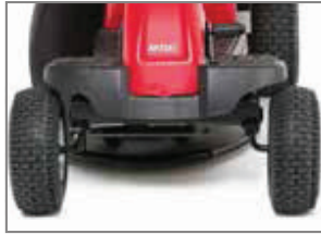
Laterally displaced deck allows mowing close to edges
