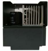
Insolated cooling air duct
