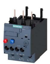
Overload relay 3.5...5.0 A Thermal For motor protection Size S0, Class 10 Contactor mounting Main circuit: Screw Auxiliary circuit: Screw Manual-Automatic-Reset
