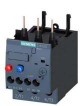
Overload relay 20...25 A Thermal For motor protection Size S0, Class 10 Contactor mounting Main circuit: Screw Auxiliary circuit: Screw Manual-Automatic-Reset
