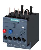
Overload relay 1.8...2.5 A Thermal For motor protection Size S00, Class 10 Contactor mounting Main circuit: Screw Auxiliary circuit: Screw Manual-Automatic-Reset
