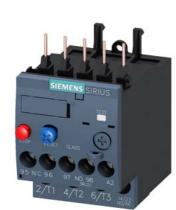
Overload relay 5.5...8.0 A Thermal For motor protection Size S00, Class 10 Contactor mounting Main circuit: Screw Auxiliary circuit: Screw Manual-Automatic-Reset
