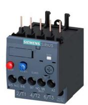
Overload relay 3.5...5.0 A Thermal For motor protection Size S00, Class 10 Contactor mounting Main circuit: Screw Auxiliary circuit: Screw Manual-Automatic-Reset
