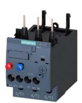
Overload relay 1.8...2.5 A Thermal For motor protection Size S0, Class 10 Contactor mounting Main circuit: Screw Auxiliary circuit: Screw Manual-Automatic-Reset
