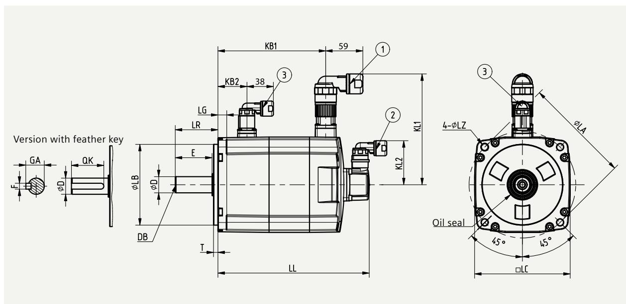
Note: ① Power connector, ② Absolute encoder connector, ③ Brake connector
