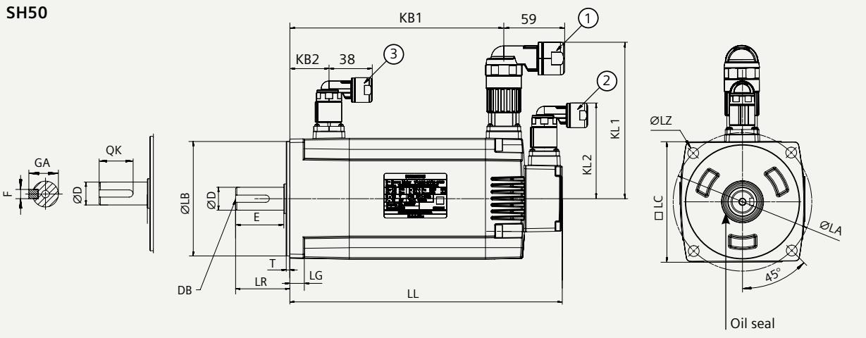
Note: ① Power connector, ② Incremental encoder connector, ③ Brake connector
