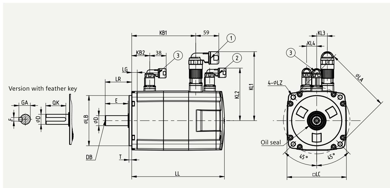
Note: ① Power connector, ② Incremental encoder connector, ③ Brake connector
