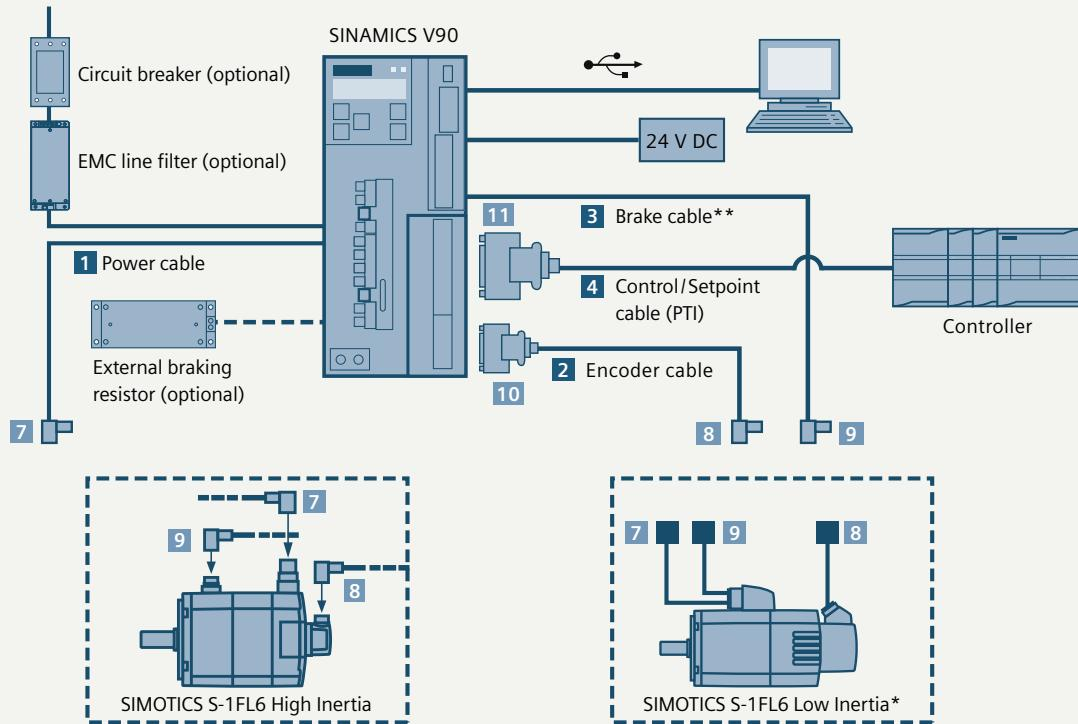
System connection diagram of SINAMICS V90 PROFINET version
