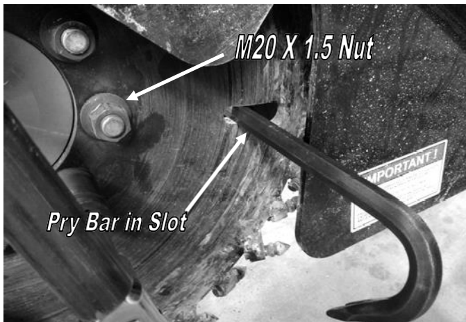
Cutter Head Lug Nut Removal
