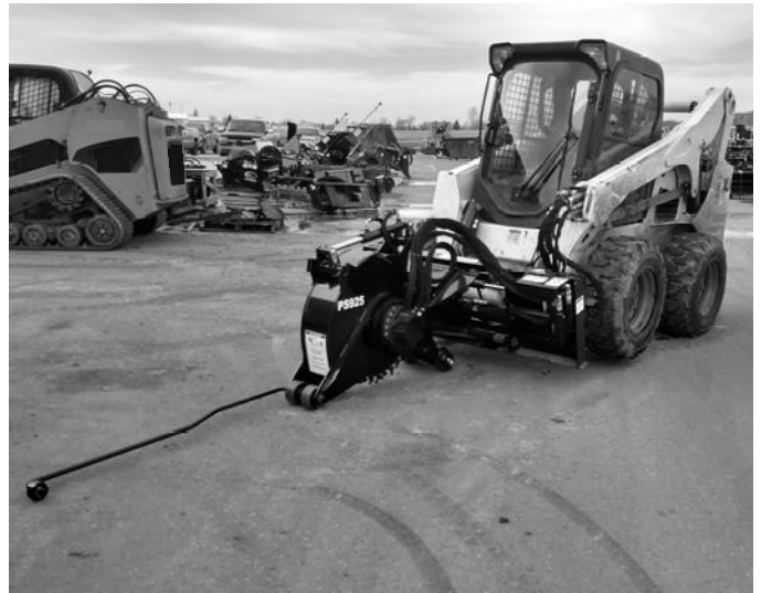
Proper Precut Position
