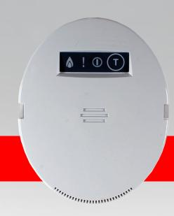
For detection of compressed natural gas (methane) in the protected area. The status is indicated with LEDs and built-in sounder. EN50194-1 compatible on trigger level 5100 ppm CNG (methane) in air, saturation 10% LEL (Low Explosion Level) of the protected area. The signal loop interface line is compatible with the IFS7002 fire control panel.
