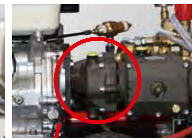
Reduction gear for reduction of pump speed (reduction gear ratio 1: 2.2)
