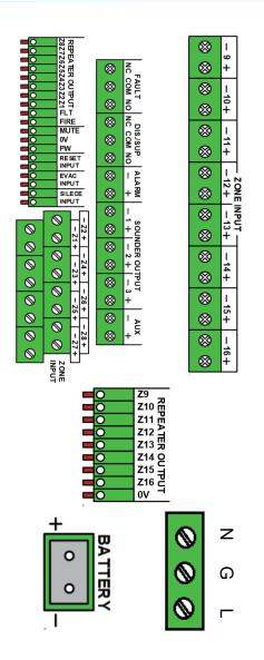
FAULT (NC, COM, NO): Fault output terminal.
