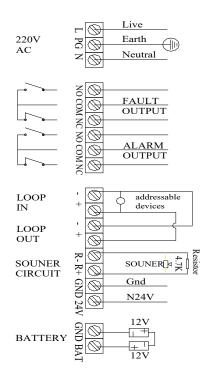
L, PG, N: 230VAC mains supply BAT, GND: 24VDC battery input
