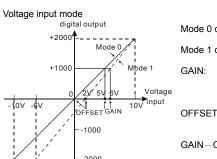
Mode 0 of CR#1: GAIN=5V(1000<sub>LSB</sub>), OFFSET=0V (0<sub>LSB</sub>). Mode 1 of CR#1: GAIN=6V(1200<sub>LSB</sub>), OFFSET=2V (400<sub>LSB</sub>).
