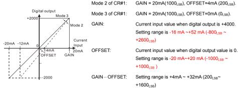
Use the chart above to adjust A/D conversion characteristic curve of voltage input mode and current input mode. Users can adjust conversion characteristic curve by changing OFFSET values (CR#18~CR#21) and GAIN values (CR#24~CR#27) depend on application
