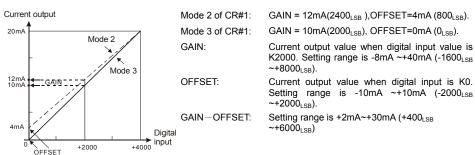
Use the chart above to adjust D/A conversion characteristic curve of voltage output mode and current output mode. Users can adjust conversion characteristic curve by changing OFFSET values (CR#14~CR#15) and GAIN values (CR#18~CR#19) depend on application.
