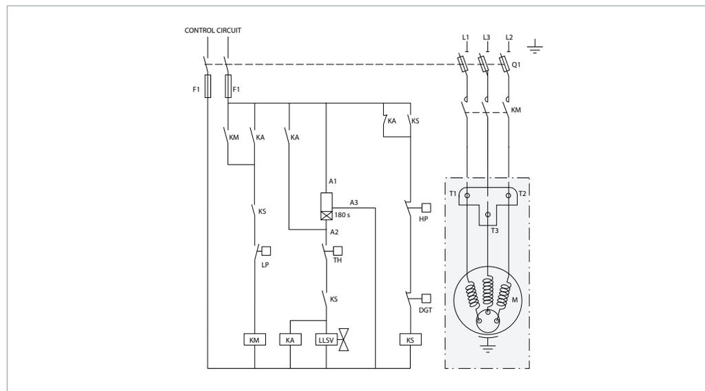
**Wiring diagram without pump-down cycle**
