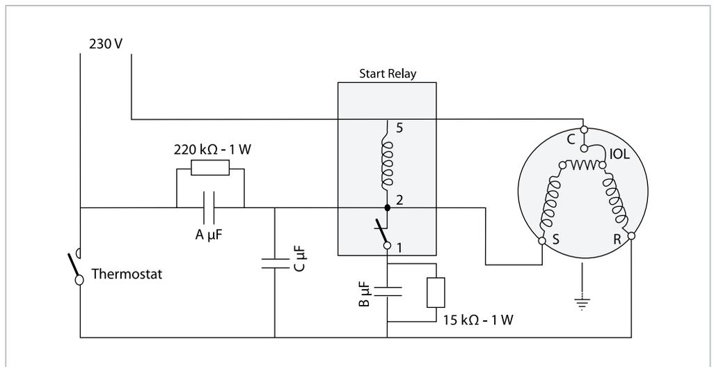
**Single phase CSR wiring without trickle circuit**
