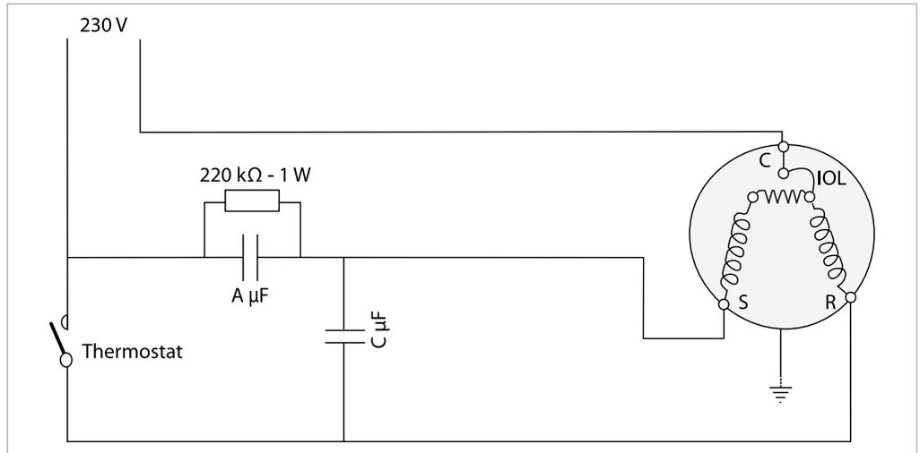
**Single phase CSR wiring with trickle circuit**
