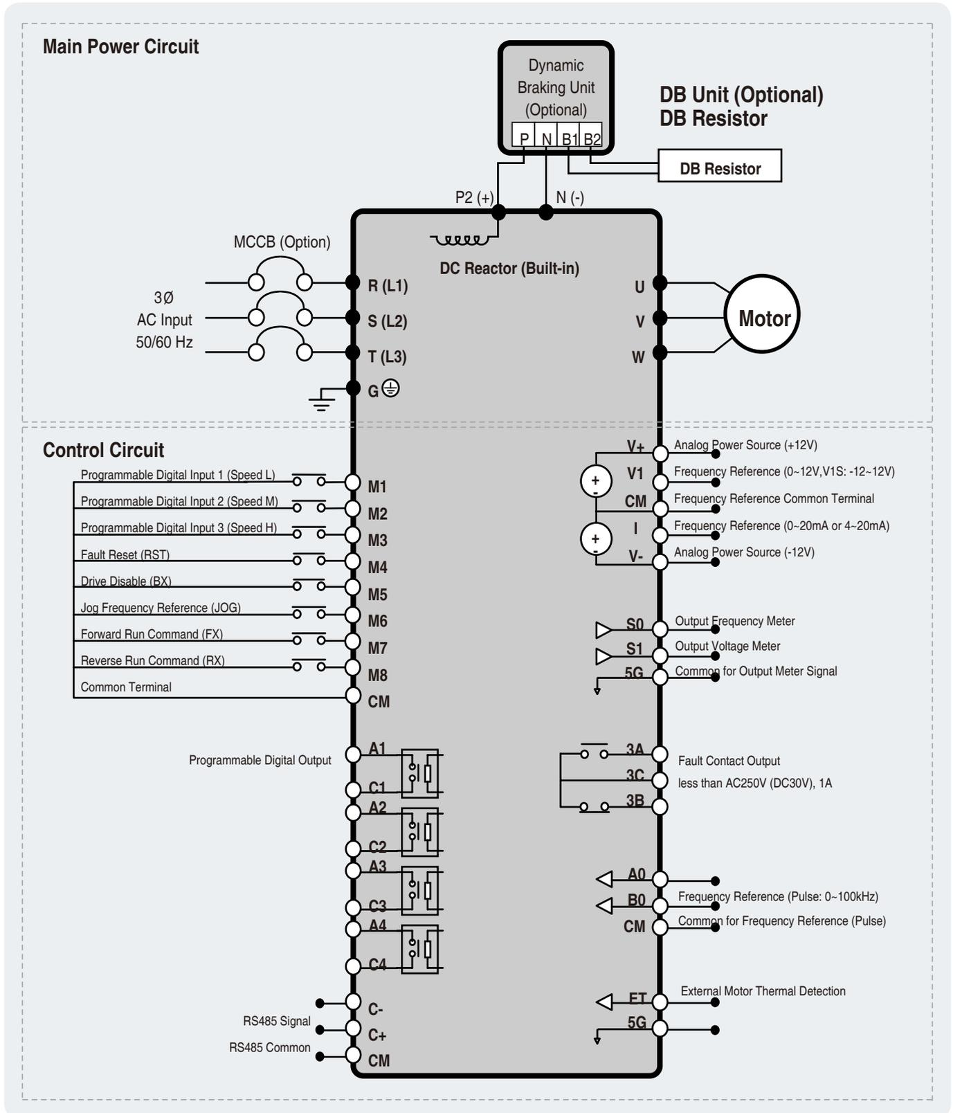
Note 1) 5G is Common Ground for Analog Meter Output (S0, S1) and External motor thermal detection (ET). CM is Common Ground for Analog input.
