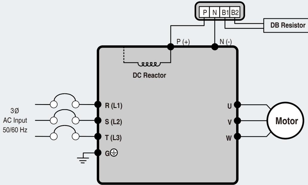
■ For 37~90kW (50~125HP) Built-in DCL Type
