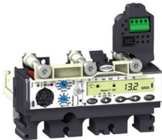
Micrologic built-in LCD display.
