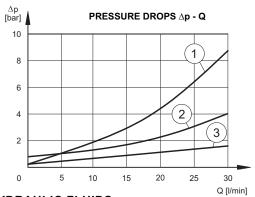
Typical  $\Delta p$  - Q curves obltained with QTM2-D valve, with throttling axis at full retraction.
