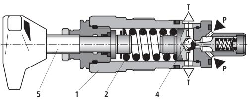
**Type DBDH 10 K1X/...** Version pressure rating 630 bar (ball seat valve, only NG10)
