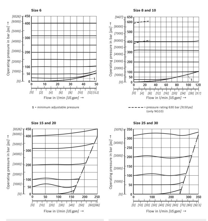
► The characteristic curves refer to the specified pressure ratings (e.g. 200 bar). The more the set pressure value differs from the nominal pressure rating (e.g. < 200 bar), the larger the pressure increase with increasing flow gets.
