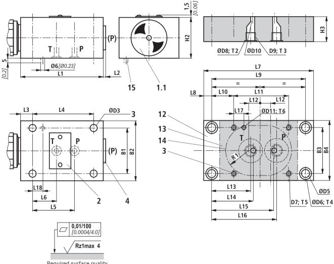
Required surface quality of the valve contact surface
