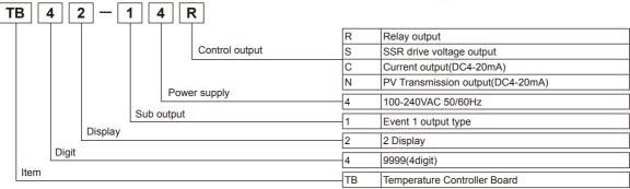
XPV transmission output type does not have Event 1 output.
