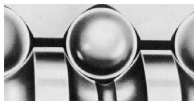
Figure 2: Ball screw groove profile
